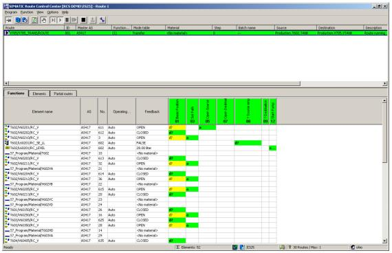
The upper part of the RCC window shows the information about a route. The lower part shows the respective route elements.
