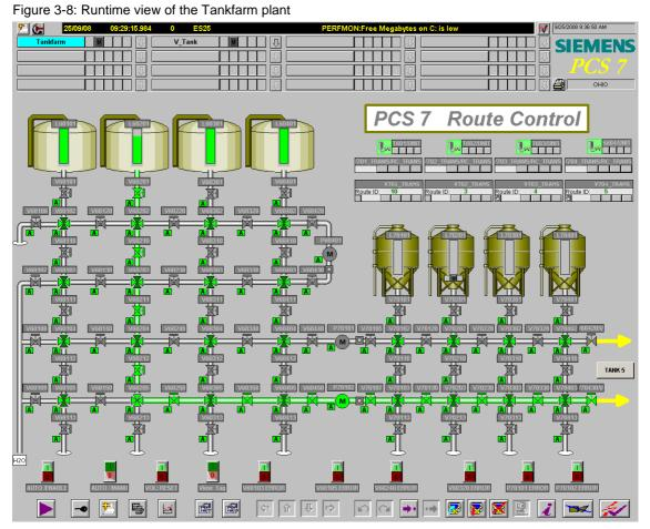
The entire plant should be in automatic mode. Thus the RC will open or activate the elements required for route selection, such as valves and motors, as soon as this is required. For this purpose the automatic mode switch must be set to "Auto".
