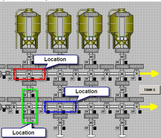
A location comprises all elements which, in the deactivated state, come into contact with the transport material.
